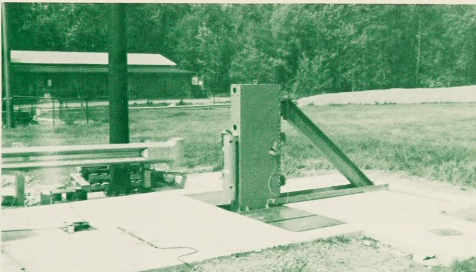
Figure 5. — Rigid instrumented pole.
