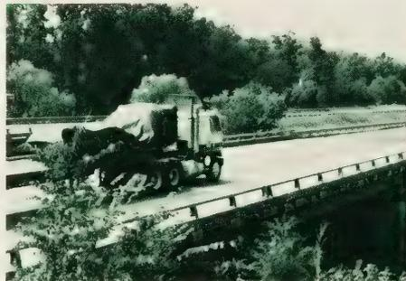
improvements in system software and hardware, weighing can be performed automatically with no traffic observer necessary. The accuracy of the in-motion weighing has been established by repeatability tests and by comparison with static weigh stations.
