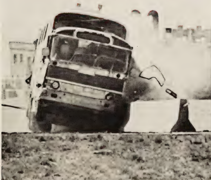
Heavy vehicle barrier test. (2)
