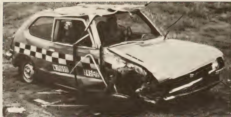
Figure 10.—Honda Civic after 60 mph (97 km/h), 15° impact with New Hampshire bridge rail.
