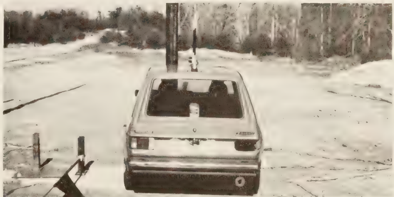
Figure 16. —Alignment of current specification breakaway pole for 60 mph (97 km/h), 1,850 lb (0.84 Mg) vehicle test.
