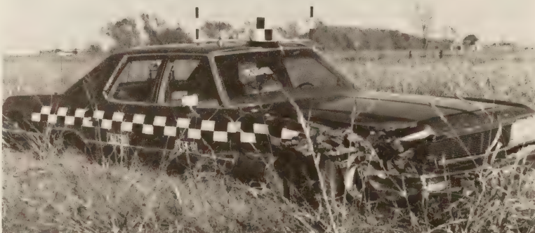
Figure 13.—Plymouth after 60 mph (97 km/h), 15° impact with New Hampshire bridge rail.
