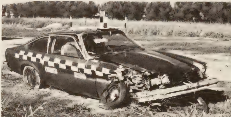
Figure 12.—Vega after 60 mph (97 km/h), 15° impact with New Hampshire bridge rail.
