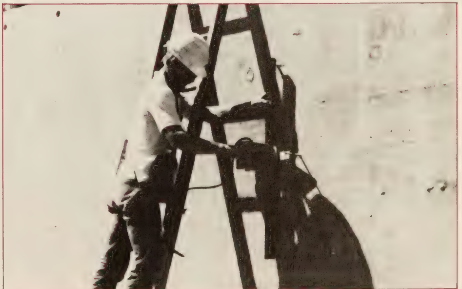
Figure 4.—(a) Tiltmeter used to monitor abutment tilt from foundation settlement. (b) Optical settlement monitoring of bridge abutment wall supported by spread footing.
