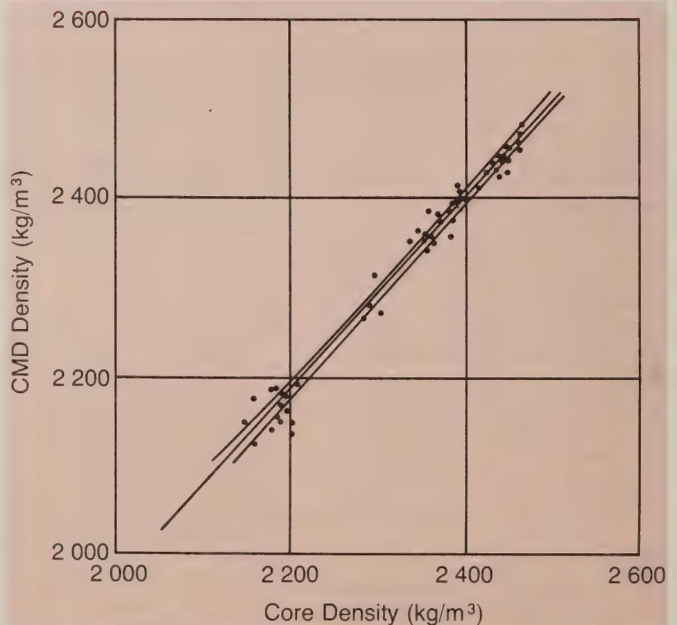
Figure 4.—Correlation between CMD density and core density measurements, laboratory static and dynamic tests (regression line and 95 percent confidence limits).
