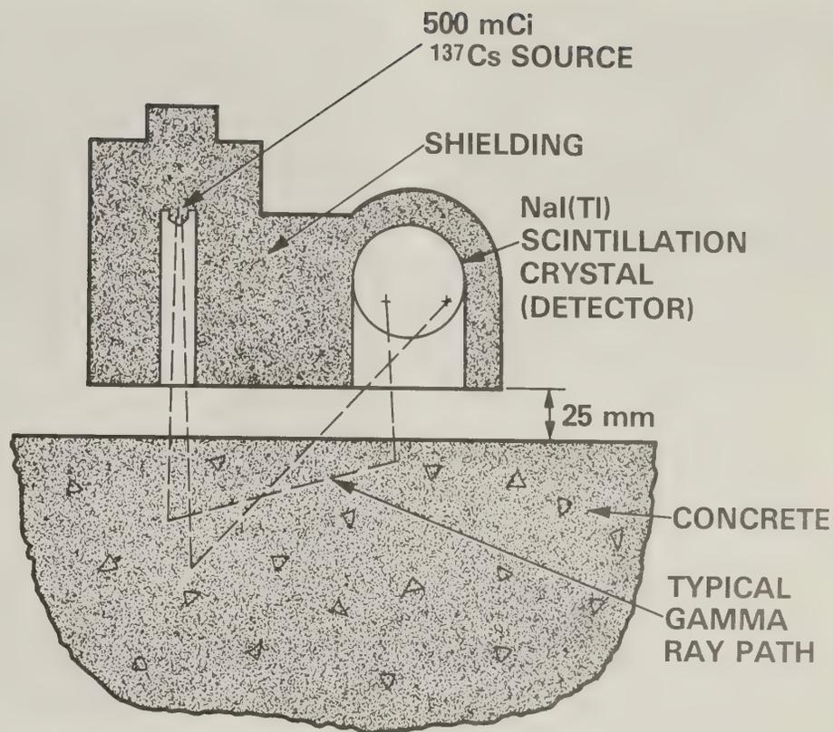
Figure 1.—Backscatter measurement with CMD source/sensor unit.
