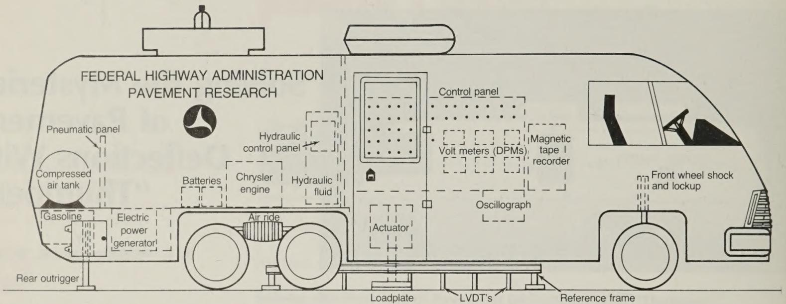
Figure 1.—FHWA pavement deflection test system.
