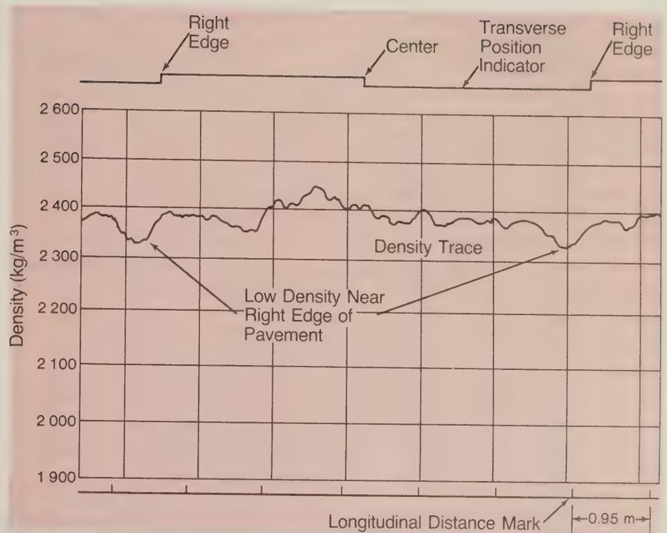
Figure 5.—Typical density trace, source/sensor unit traversing pavement.
