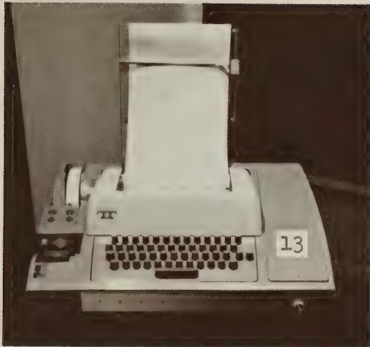
Figure 3.—Teletype used by the operator to communicate with the system's processor.
