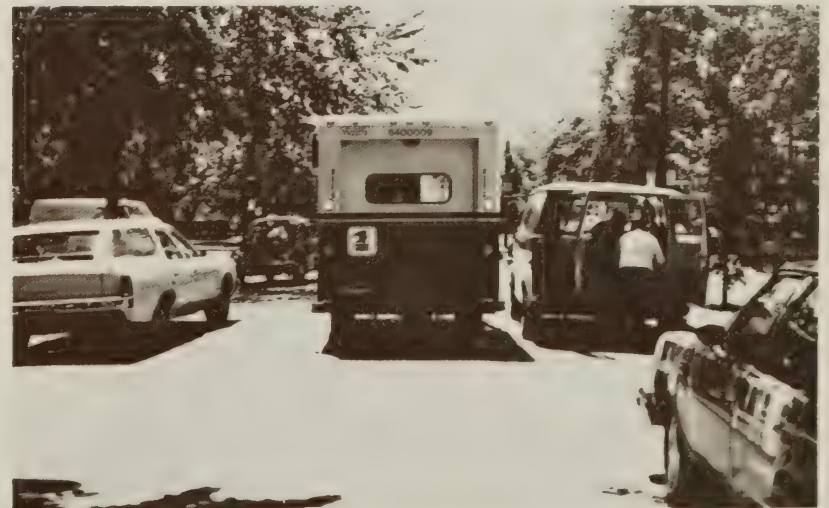
Figure 2.—Double parked mail truck causes through traffic to move to far left lane.
