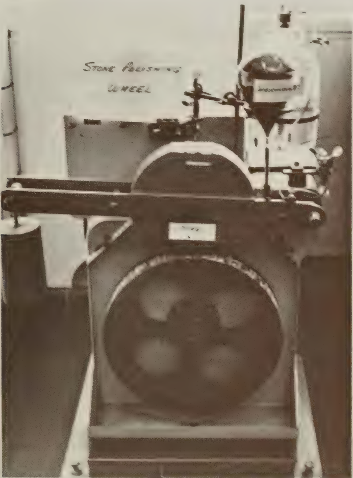
Figure 7.—The British wheel apparatus used for testing aggregate polish susceptibility.
