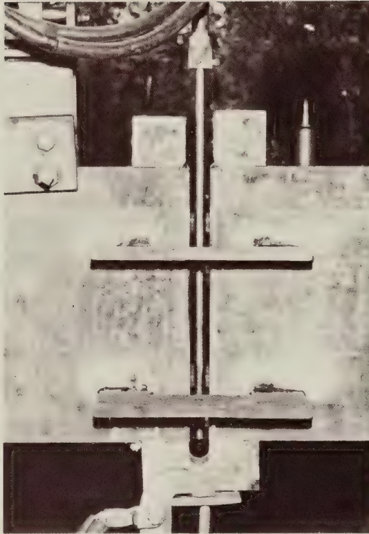
Figure 1b.—Electroslag joint preparation showing strong-backs, starting sump, run-off tabs, consumable guide tube, and spacer ring.
