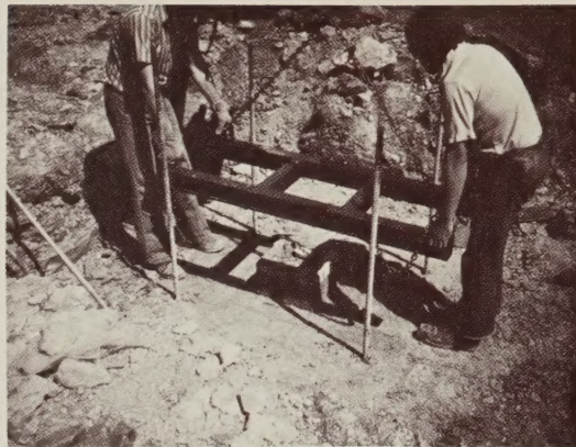
Lower frame of testing device being positioned over sawed specimen.
