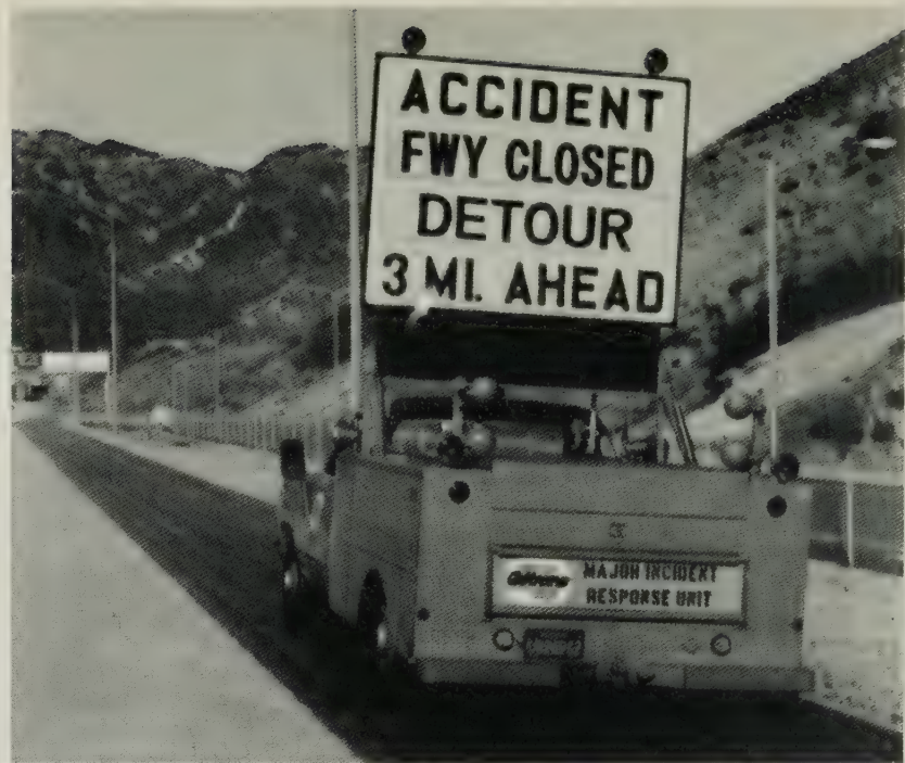
Figure 9.—Traffic messages are quickly developed with fabric signs used by the California incident response teams.
