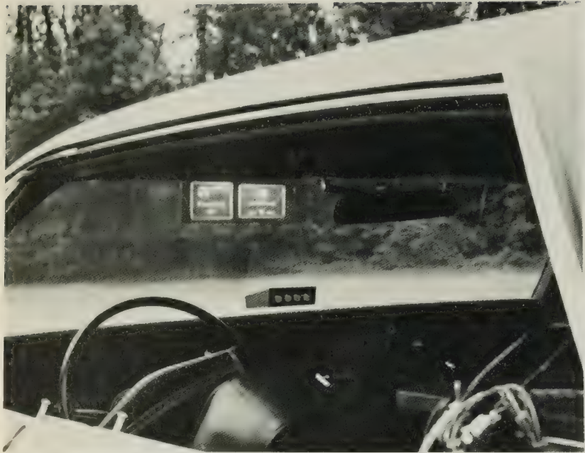
Figure 1.—Subject response lamps on dashboard and projection screen on windshield.
