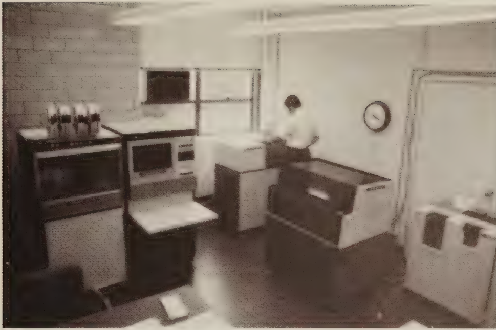
Figure 1.—A remote terminal used to enter batch programs to the central computer site.
