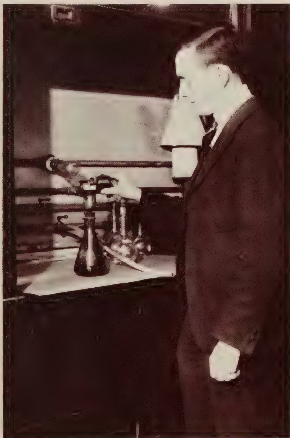
Figure 1.—The BPR laboratory about 1915. Apparatus for determining bitumen content is essentially same today as then; however, trichloroethylene is used instead of carbon disulfide because of fire hazards with carbon disulfide.
