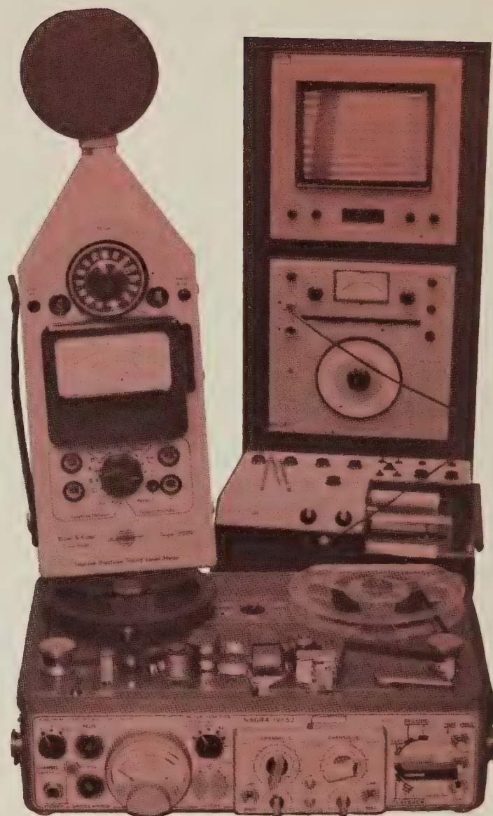
A. Precision sound level meter, with windscreen B. \frac{1}{3} band octave analyzer and level recorder C. Tape recorder
