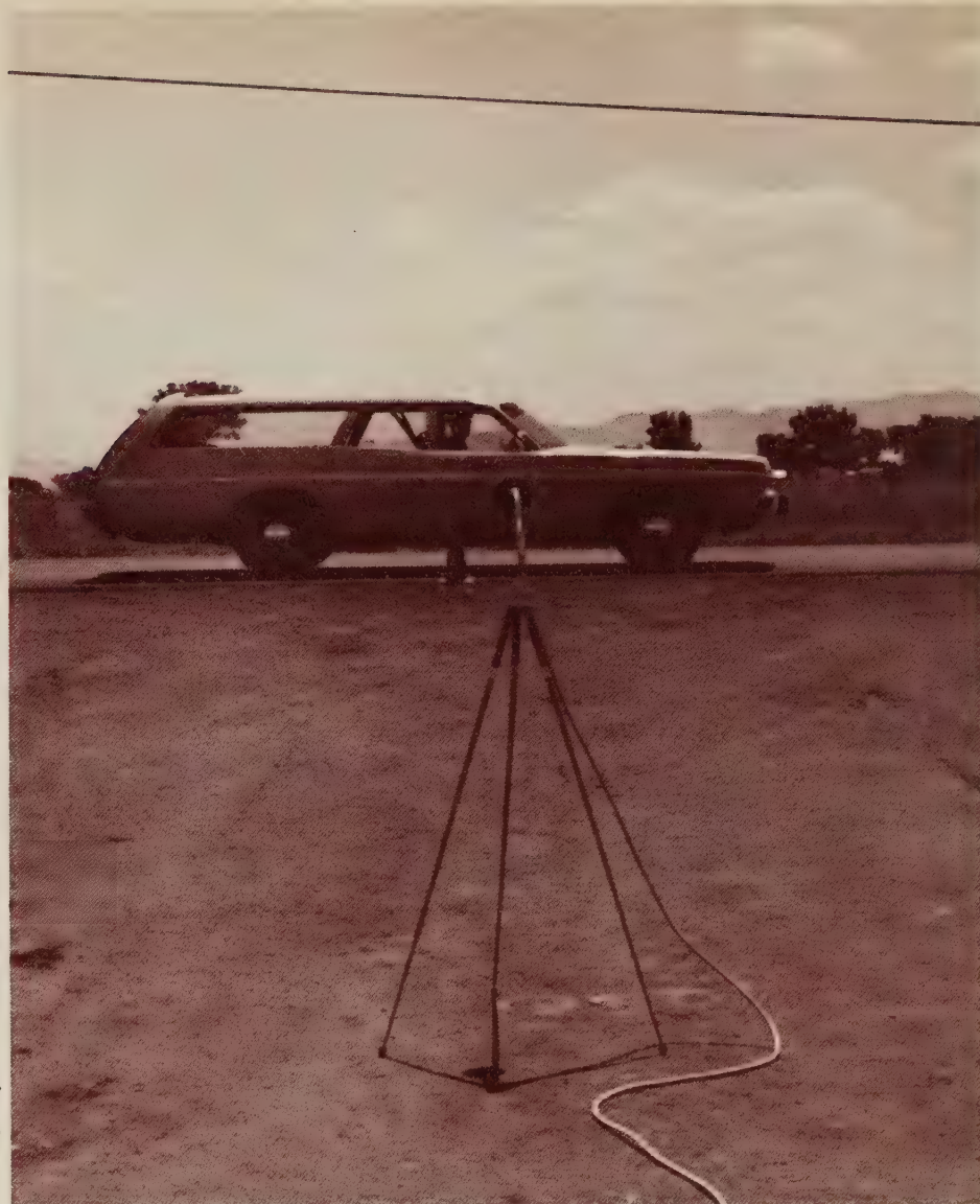
Test vehicle at midpoint of test course with tripod-mounted microphone 50 ft from edge of lane.
