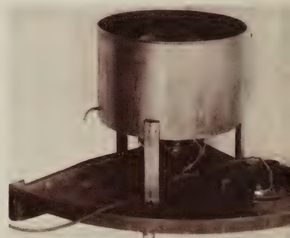
Figure 4.—One of the original asphalt extractors used in the BPR laboratory. The inverted bowl was a BPR innovation and was used by BPR for a number of years.
