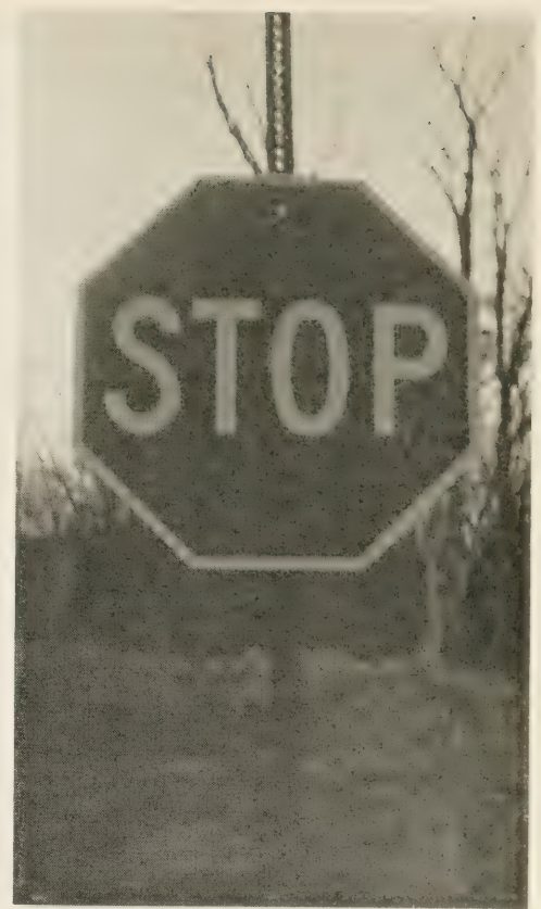
Figure 2.—STOP sign—an example of redundancy.
