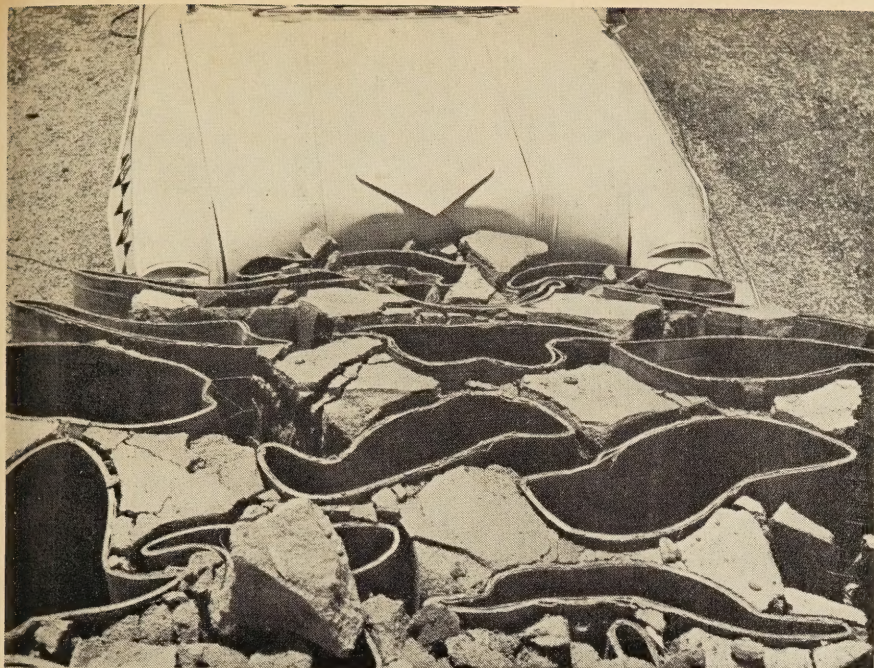
A cardboard-concrete barrier design—a “safe” vehicle impact.
