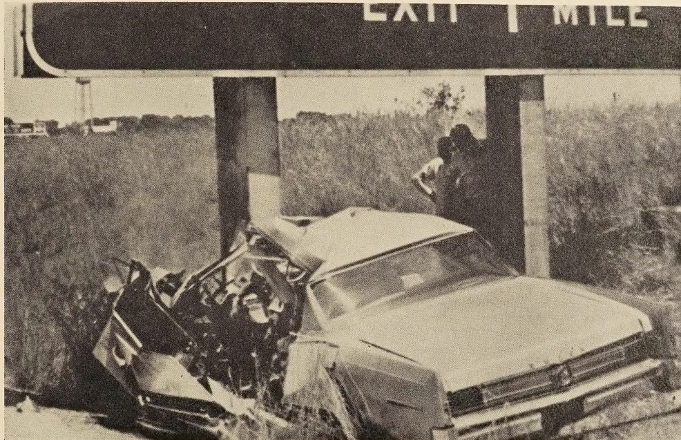
Figure 6.—Collision with a rigid sign post—a fatal accident.
