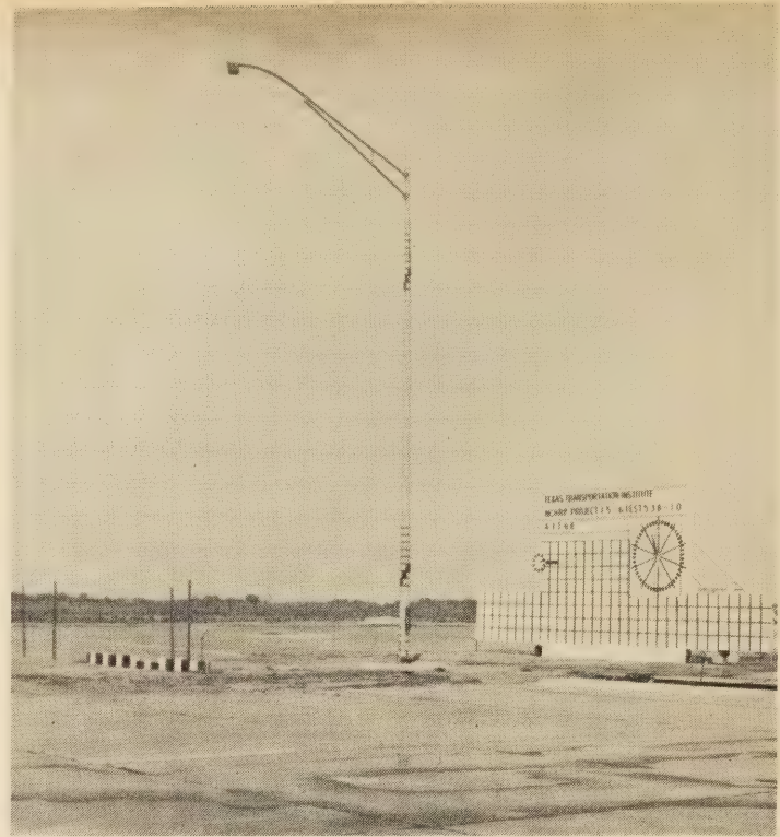
Figure 11.—Slip-base luminaire installation.
