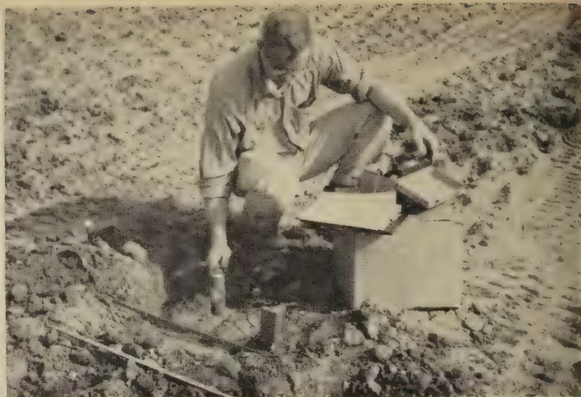
Rapid testing on 6-inch silty-gravel compacted base course. Above left—Plate-bearing test using truck-mounted, hydraulically actuated equipment. Above right—Refraction seismographic test.
