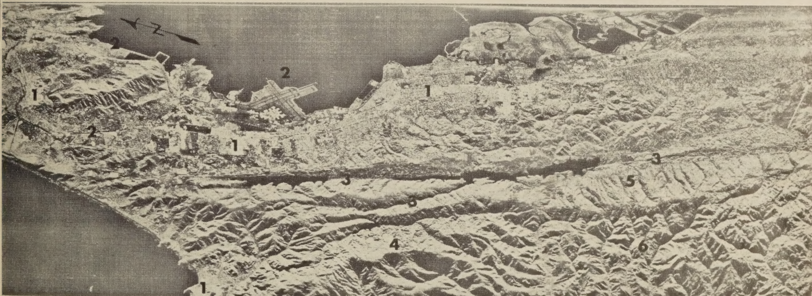
Figure 1.—Radar image of portion of San Francisco peninsula illustrating regional view obtained by side-looking radar and its ability to distinguish numerous features important to highway planning. Numbered items are discussed in text. 2
