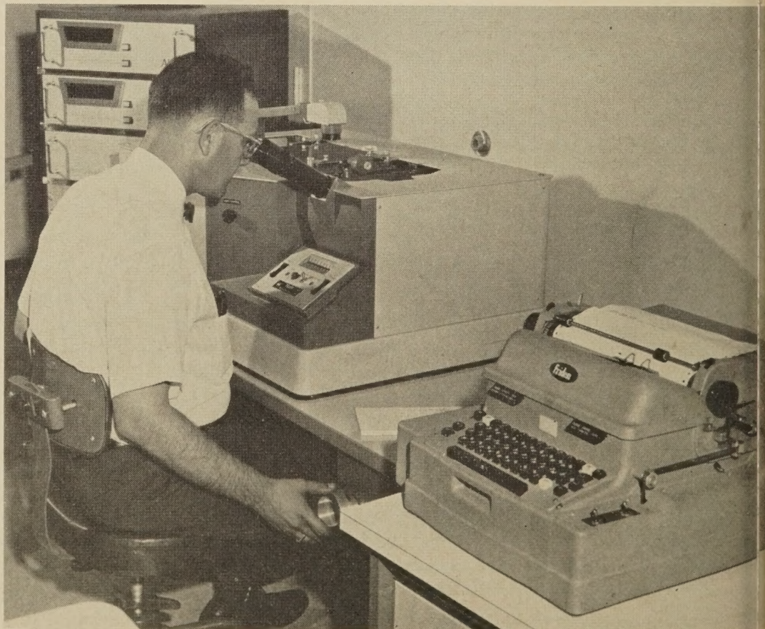
Figure 2.—Nistri monocomparator, model TA1/P and accessory equipment.
