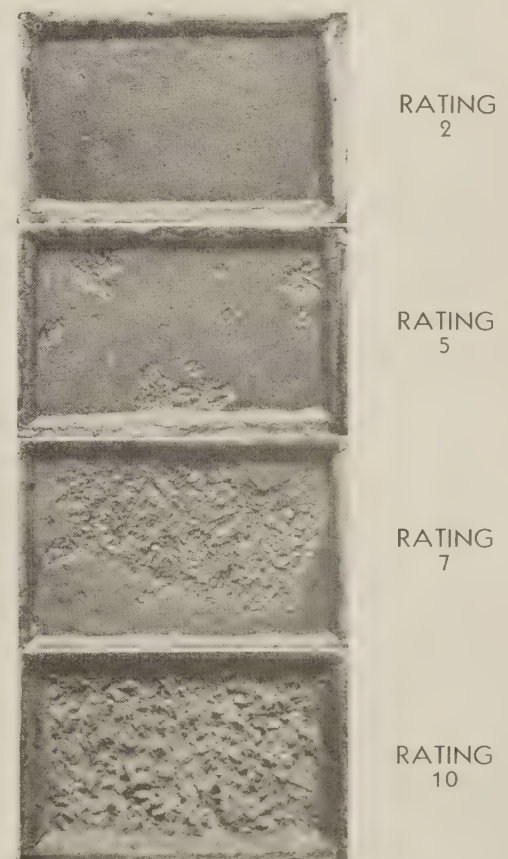
Figure 2.—Examples of typical ratings used to evaluate surface scaling of specimens subjected to outdoor freezing and thawing by calcium chloride.
