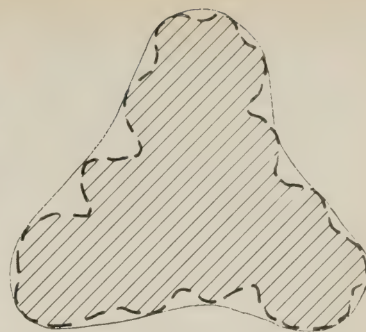
Figure 1.—Characteristic outline of tri-n-propylamine cation model is represented by dashed line. The relaxed, solid outline was used to measure the cross-section area of the cation.
