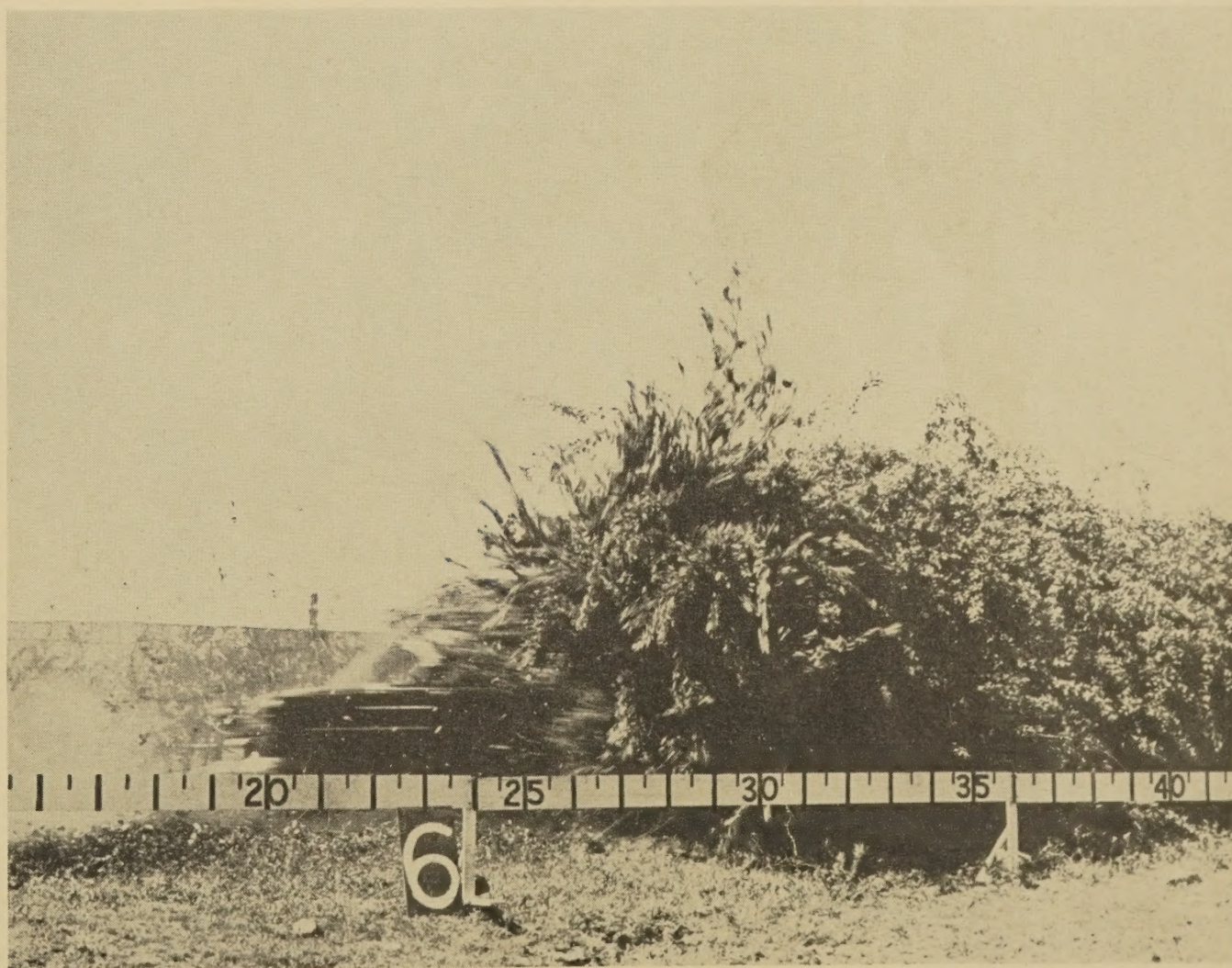
Testing the effectiveness of multiflora rose hedges as a crash barrier.
