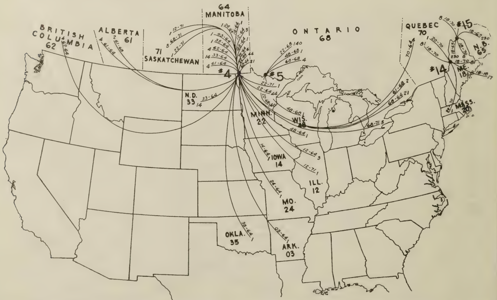
Figure 6.—Origin and destination and number of trips made by commercial vehicles crossing the border at stations 4, 5, 14, and 15 on an average summer weekday in 1954.
