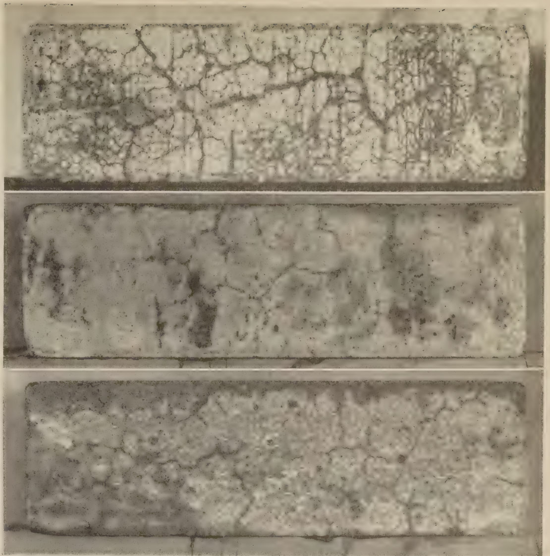
Figure 3.—Abnormal expansion of specimens containing sand-gravel aggregate: (top) grading 1 with cement 1, at end of cycle C; (center) grading 2 with cement 1, at end of cycle E; (bottom) grading 1 with cement 3, at end of cycle E.
