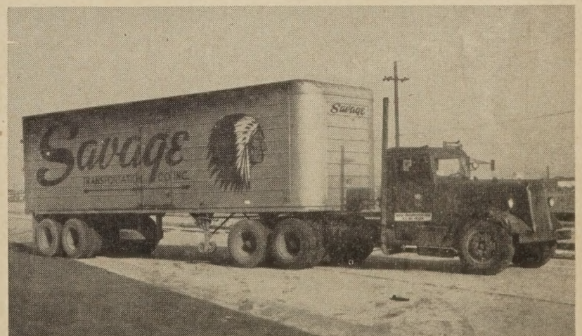
A five-axle combination vehicle, popular in the western part of the country.
