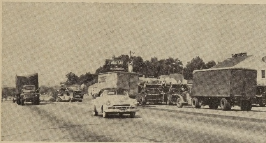
East of the Rockies, about one-third of the commercial vehicles (exclusive of light trucks) are three- and four-axle tractor-truck semitrailer combinations. They carry two-thirds of the tonnage hauled, and are responsible for almost all of the heavy axle loads.
