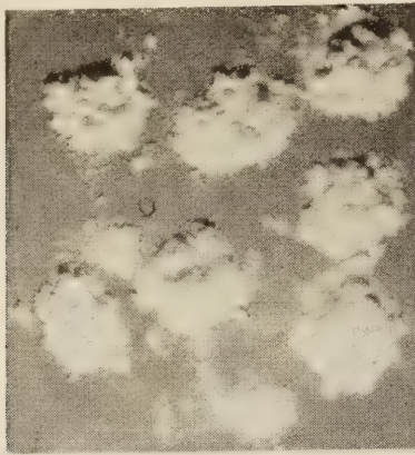
Figure 8.—EXTENT OF REACTION PRODUCT DEVELOPED BETWEEN A POROUS SANDSTONE AND CEMENT CONTAINING AN AVERAGE OF 0.92 PERCENT TOTAL ALKALIES, AFTER 9 WEEKS' STORAGE IN CAUSTIC SOLUTION.
