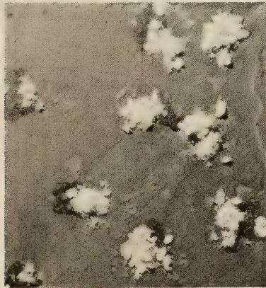
Figure 6.—REACTION OBTAINED IN 65 DAYS WITH CEMENT CONTAINING 0.92 PERCENT TOTAL ALKALIES AND ALTERED TRACHYANDESITE, AN IGNEOUS ROCK TYPE.
