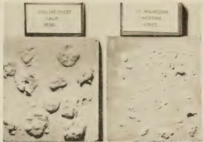
Figure 7.—REACTION OBTAINED USING OPALINE CHERT AND SILICEOUS-MAGNESIAN LIMESTONE WITH CEMENT CONTAINING 0.92 PERCENT TOTAL ALKALIES.
