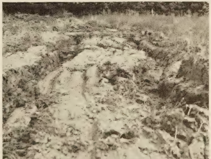
FIGURE 19.—SOFT CONDITION OF SOIL IN FILL AREA AFTER THE FLOOD WATERS RECEDED. A TRACTOR WAS MIERED AT THIS LOCATION IN INDIANA.
