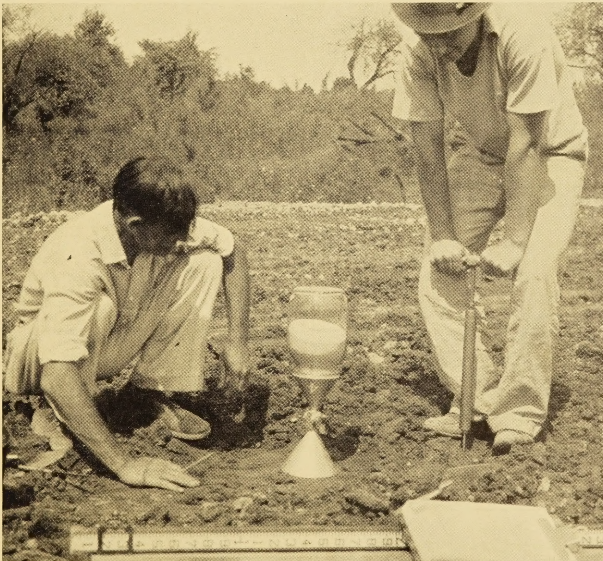
APPARATUS USED IN MAKING EMBANKMENT STUDIES
