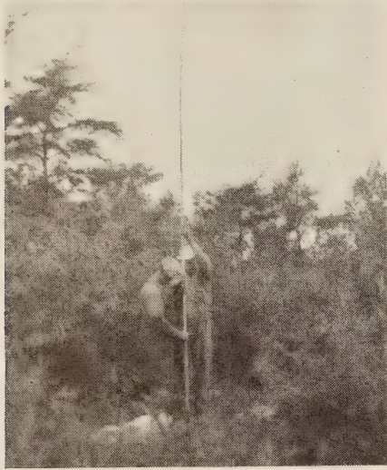
FIGURE 5.—BORING WITH A POST-HOLE AUGER TO DETERMINE THE CHARACTER OF THE SUBSURFACE MATERIALS.
