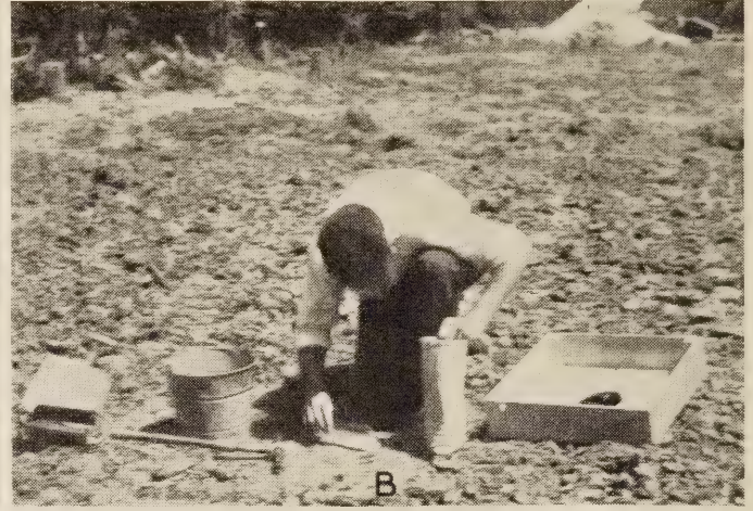
FIGURE 23.—REMOVING SOIL WITH POST-HOLE AUGER TO DETERMINE DENSITY OF COMPACTED LIFT AND DETERMINING THE VOLUME BY FILLING THE HOLE WITH SAND OF KNOWN WEIGHT PER UNIT VOLUME (INDIANA PROJECT).
