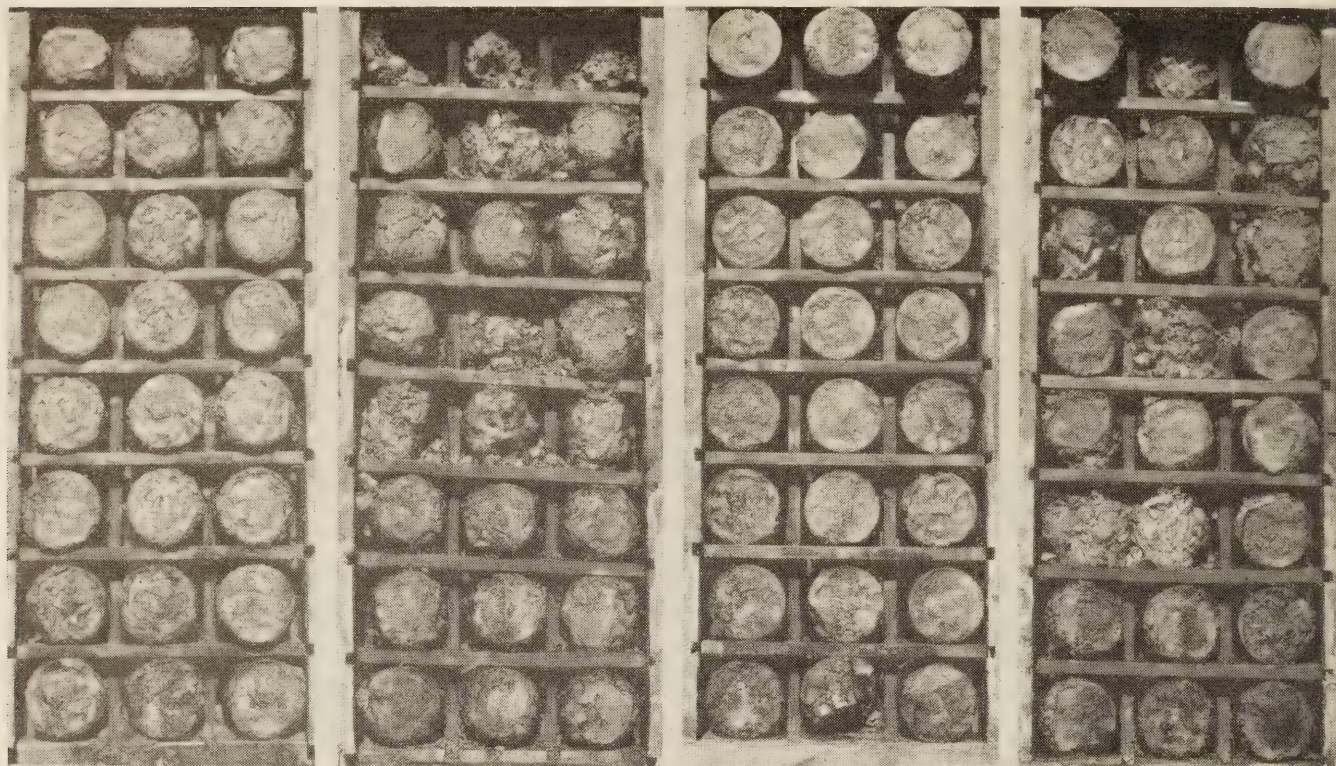
FIGURE 1.—CONDITION OF CONCRETE SPECIMENS WITH CEMENT A, AFTER 55 MONTHS IN MEDICINE LAKE. W/C RATIO=0.7. TWO TOP ROWS OF EACH CRATE IMMERSSED \frac{1}{2} HOUR, WITH EACH SUCCESSIVE LOWER TWO ROWS IMMERSSED 1 HOUR, 4 HOURS, AND 24 HOURS IN WATER-GAS TAR. DATA GIVEN IN TABLE 7.
