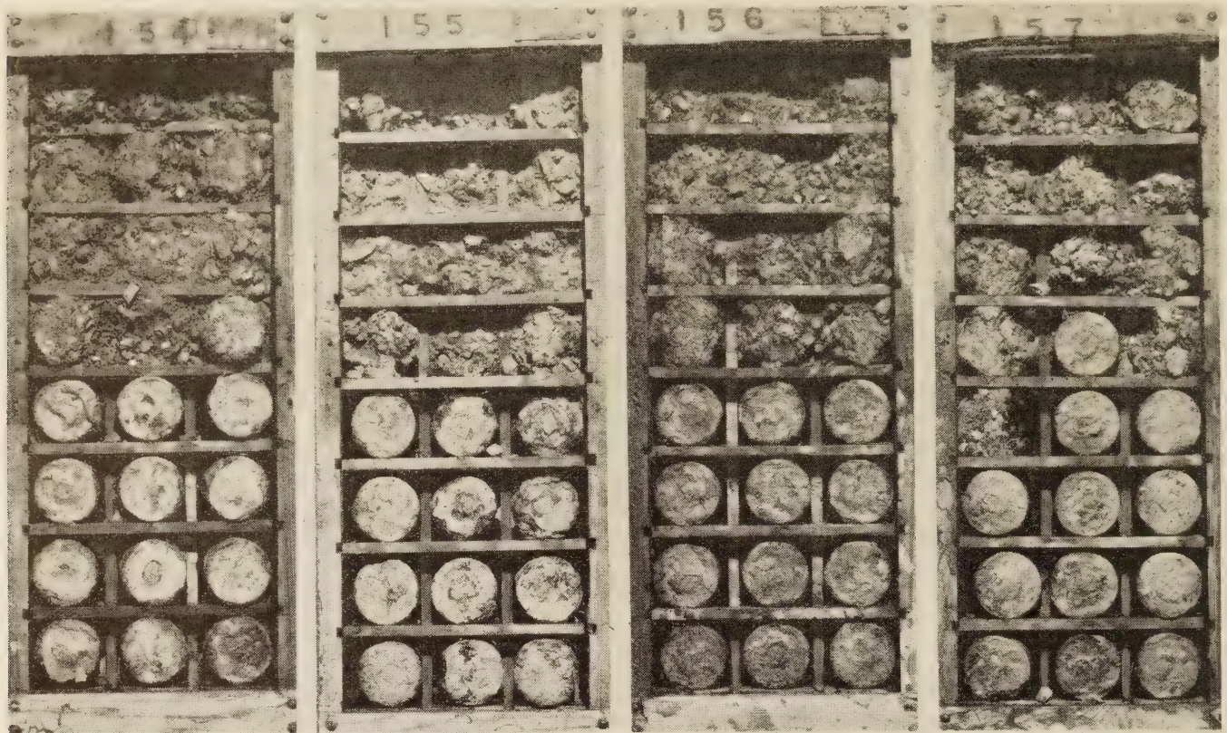
Crate No. 154 Cure, moist 7 days Cure, air 1 day 155 7 days 7 days 156 28 days 1 day 157 28 days 7 days
