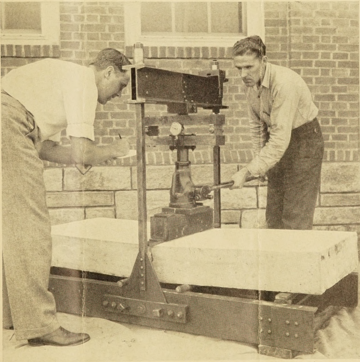
ENGINEERS MEASURE THE STRENGTH OF A MONOLITHIC BRICK TEST SLAB
