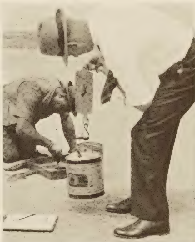
FIGURE 24.—BY DETERMINING THE WEIGHT OF OIL REMAINING IN THE CAN, THE WEIGHT AND VOLUME OF OIL REQUIRED TO FILL THE HOLE ARE DETERMINED.
