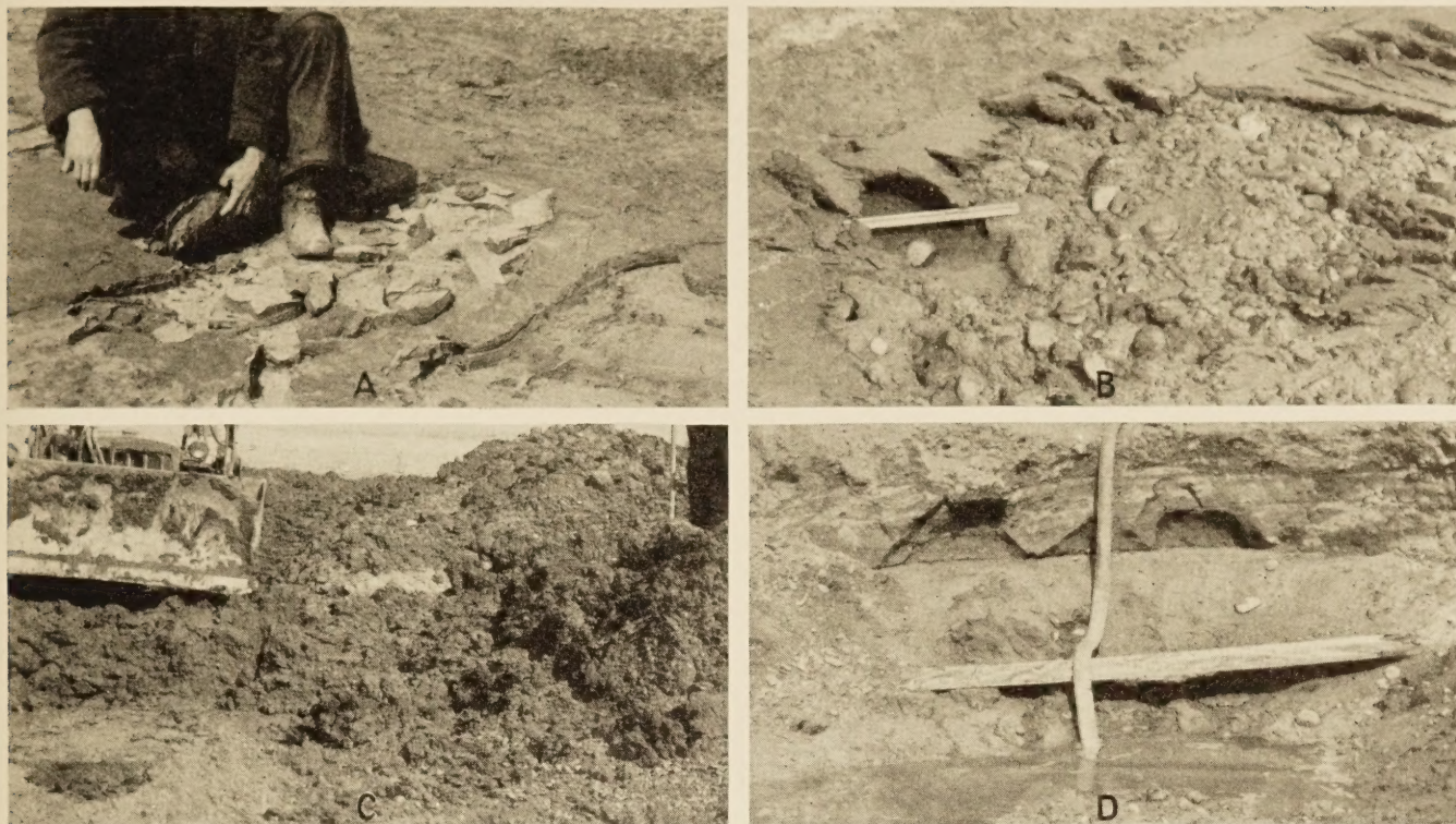
FIGURE 4.—TYPICAL EXAMPLES OF POCKETS AND LAYERS OF MUCK AND SAND. A, THIN LAYERS OF MUCK; B, POCKET OF MUCK, GRAVEL, AND ENTRAPPED WATER; C, DEEP POCKET OF SOFT MUCK; AND D, SANDY DEPOSIT WITH THIN LAYERS OF MUCK.
