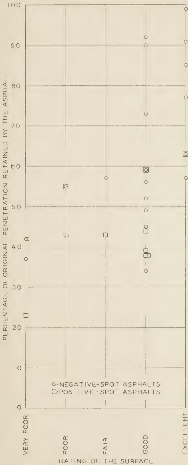
FIGURE 10.—RELATION OF SURFACE CONDITION TO PERCENTAGE OF ORIGINAL PENETRATION RETAINED BY THE ASPHALT. (ALL SAMPLES TAKEN WHERE THE BASE WAS POOR OR VERY POOR HAVE BEEN OMITTED.)
