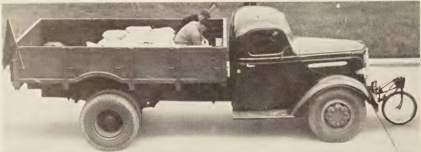
FIGURE 2.—TRUCK EQUIPPED WITH CHRONOGRAPH AND BICYCLE WHEEL AS USED IN GRADE ABILITY DETERMINATIONS.
