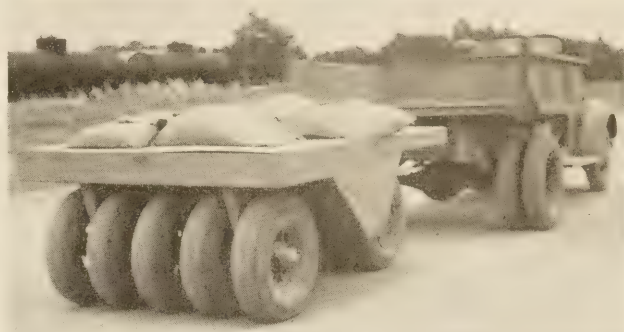
A PNEUMATIC-TIRED ROLLER ESPECIALLY DEvised TO CONSOLIDATE STABILIZED SOIL SURFACES.
