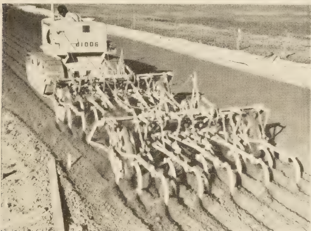
A SPRING-TOOTH HARROW WHICH PERMITS POSITIVE CONTROL OF THE DEPTH OF PENETRATION OF THE TEETH.
