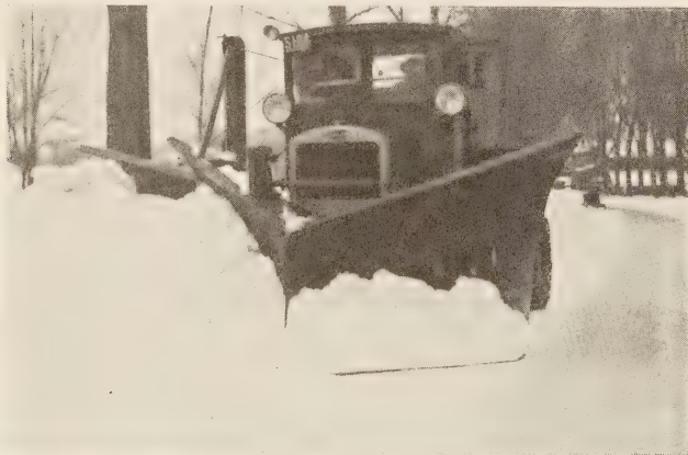
V-TYPE SNOW PLOW SUITABLE FOR MODERATELY HEAVY WORK
