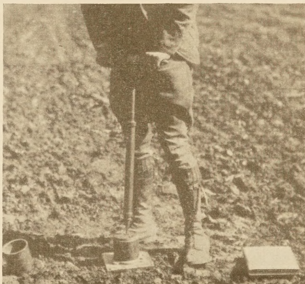
FIGURE 2.—UPPER; THE PROCTOR COMPACTION TEST APPARATUS. LOWER; MEASURING THE STABILITY OF A SAMPLE IN THE FIELD.
