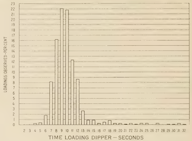
FIGURE 3.—DIAGRAM SHOWING PERCENTAGE OF LOADING OPERATIONS PERFORMED IN VARIOUS TIME INTERVALS. BASED ON 734 LOADINGS OF 1 1/4-YARD SHOVEL WORKING IN 2 1/2 TO 7 FEET OF CLAY WITH A FEW BOULDERS.
