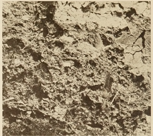
FIGURE 3.—CHARACTER OF MUCK ENCOUNTERED. MATERIAL AT THIS SPOT DISTURBED WITH DYNAMITE IN EFFORT TO HASTEN DOWNWARD PERCOLATION INTO UNDERLYING SAND LAYER
