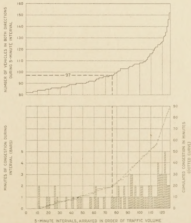
FIGURE 5.—DETERMINATION OF TRAFFIC CAPACITY OF 2-LANE ROADS, 60 PER CENT OF TRAFFIC IN ONE DIRECTION
