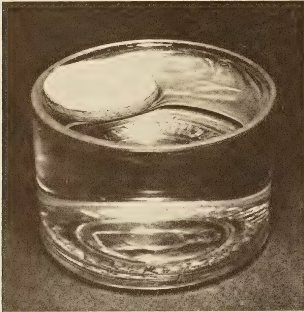
FIGURE 64.—DRIED PAT OF DIATOMACEOUS EARTH (SAMPLE 13, TABLE 15) FLOATING IN WATER AFTER BEING COATED WITH SHELLAC. APPARENT SPECIFIC GRAVITY LESS THAN ONE
