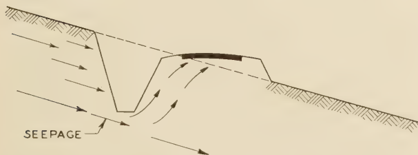
B - HIGHWAY ON SIDE-HILL LOCATION
