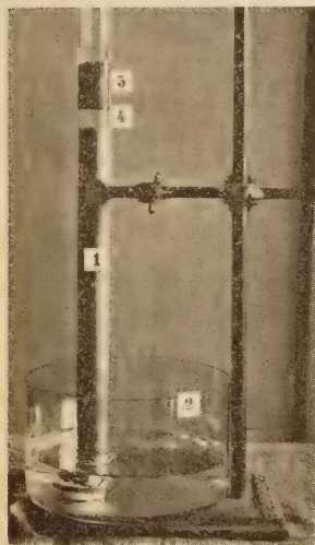
FIGURE 4.—APPARATUS USED IN DEMONSTRATING ACTION OF CAPILLARY WATER IN DRIVING AIR FROM PORES OF SOIL
