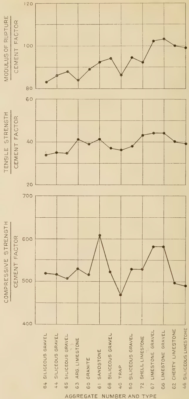
FIGURE 11.—RELATION BETWEEN CEMENT FACTOR AND FLEXURAL, TENSILE, AND COMPRESSIVE STRENGTHS, AVERAGE OF ALL TESTS
