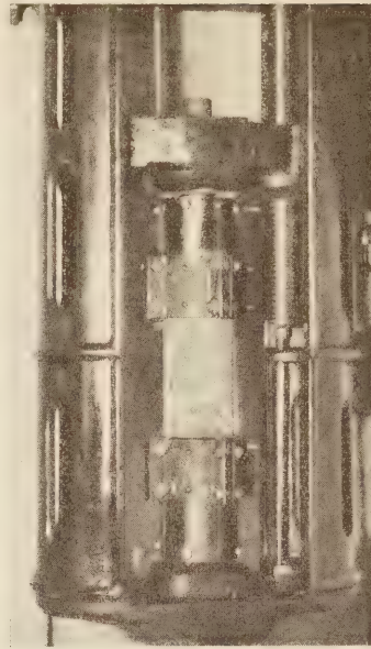
FIGURE 2.—A TENSION SPECIMEN READY FOR TESTING
