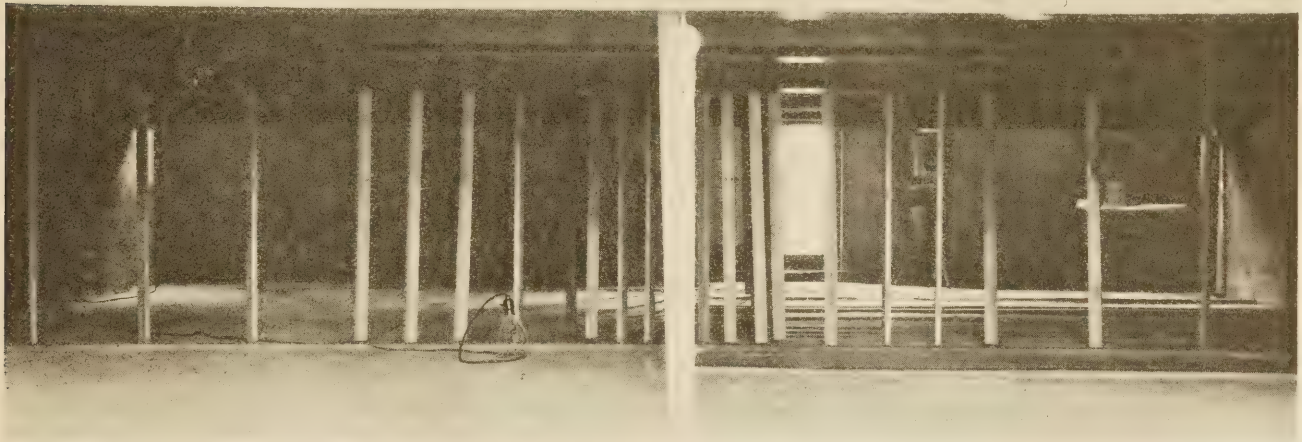
FIG. 31.—WOODEN RODS IN PLACE FOR THE MEASUREMENT OF DEFLECTIONS OF SECOND TEST SLAB
