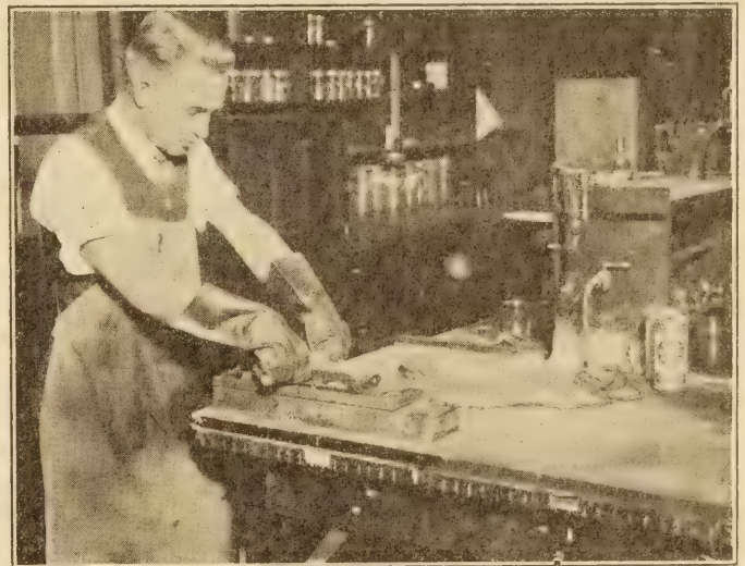
FIG. 2.—MOLDING BRIQUETTES, USING THE APPARATUS FOR CONTROL OF PRESSURE
