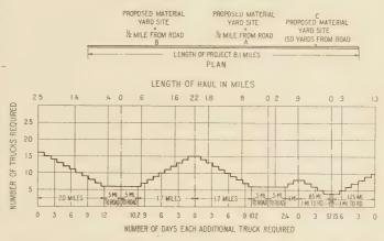
FIG. 5.—Relation of location of material yard to truck supply required (see figs. 3 and 4). If the contractor had hauled from the three sites shown, the cost of hauling would have been reduced to the lowest possible level
