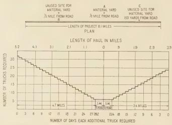
Fig. 3.--Relation of location of material yard to truck supply required. This set-up was actually used by the contractor
