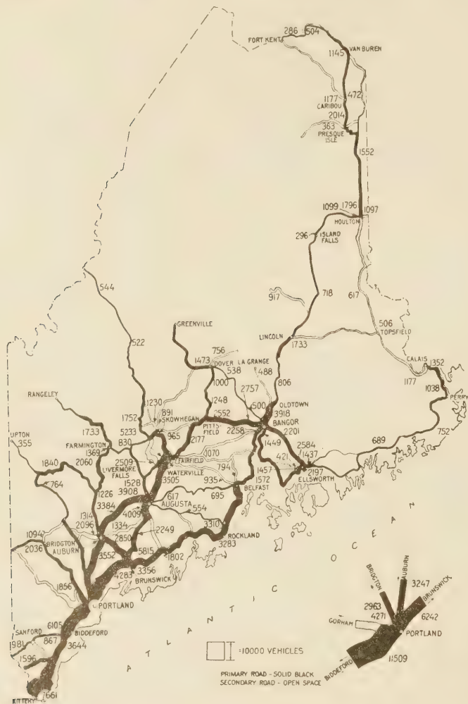
FIG. 10.—Anticipated density of traffic on primary and secondary highway systems of Maine, July to November, 1930
