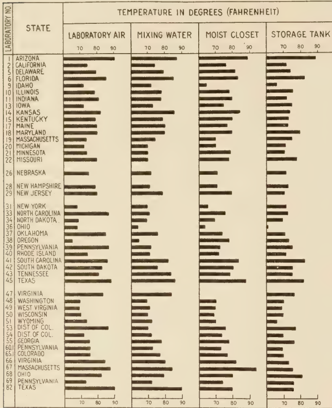
Temperatures reported in check tests of cement sample Ct-5
