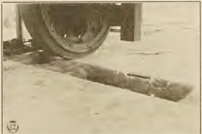
Set-up for the corner test. Strain gauges on top of slab are for determination of maximum tensile stress. Those in edge of slab locate the neutral plane.
