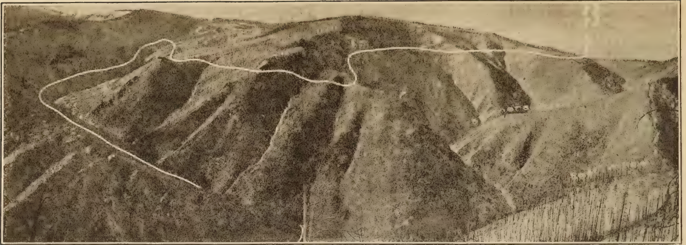
SHOWING RECONNAISSANCE SURVEY OF THE ALTERNATE ROUTES FOR THE WHEELER NATIONAL MONUMENT TRAIL THROUGH THE BURNED-OVER REGION RIO GRANDE NATIONAL FOREST, COLORADO.
