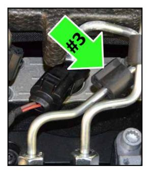
← Install fuel line dampener (03L 130) 118) in the center of #3 fuel line as shown <arrow>
