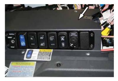
3. Inspect the rear of the mirror switch for signs of overheating. If the switch shows signs of overheating, such as wire insulation melted or discolored, replace the switch with partnumber 25165161.
