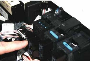
5. Lay harness into position and route towards the mirror switch located on the switch panel. Disconnect the mirror switch and can harness between the switch and cab harness.
