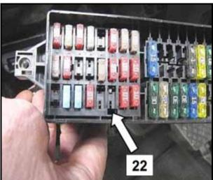
Remove fuse from position 22 of the fuse holder <arrow 22> and discard fuse
