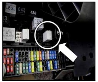
If previously equipped, reinstall the relay contact housing and reinstall relay of anti-theft system <circle> into relay carrier
