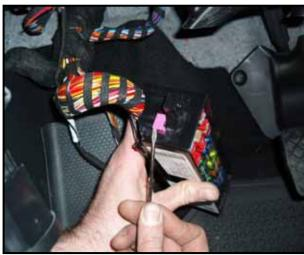
Remove the large purple secondary locking mechanism in the fuse contact housing that locks the lower half of the fuse block (fuses 17 through 60) <as shown>
