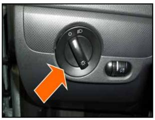
Reinstall the headlight switch <arrow> by pushing in until you hear an audible "click"
