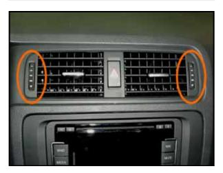
Note: Before removing the trim, ensure all left and center air vent knobs are set in the fully OPEN position (all the way up) as shown. Damage will occur if this is not done
