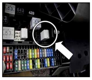
If present, pull out relay <circle> of anti-theft system from relay carrier
