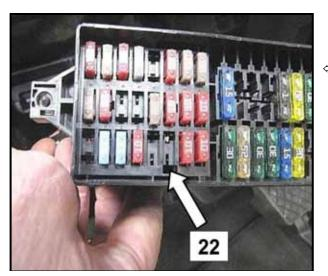
Remove fuse from position 22 of the fuse holder <arrow 22>
