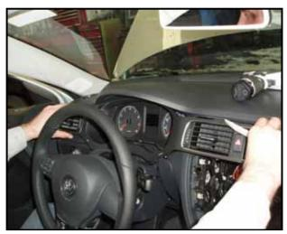
Pull out trim assembly slightly, disconnect the wiring harness for emergency lamp switch E3, then remove instrument cluster trim from the instrument panel
