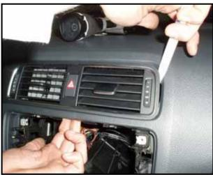
In location of center vents, push trim from behind <as shown> in order to create a gap, then using trim removal wedge 3409 or equivalent, carefully pry around trim <as shown> to loosen trim from dash panel
