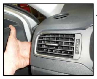
← Reach behind left vent trim panel and push trim out slightly <as shown> to loosen trim from dash panel
