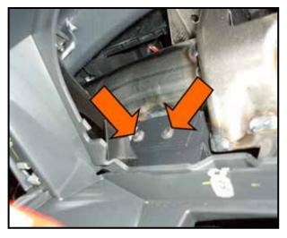
← Remove two screws <arrows> located in lower left corner area of dash panel where instrument cluster was removed
