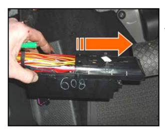
Remove the rear housing from the fuse holder by lifting both locking tabs and sliding the cover <in direction of arrow>
