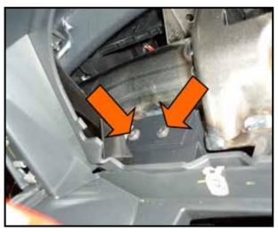
Reinstall two screws <arrows> located in lower left corner area of dash panel where instrument cluster was removed
