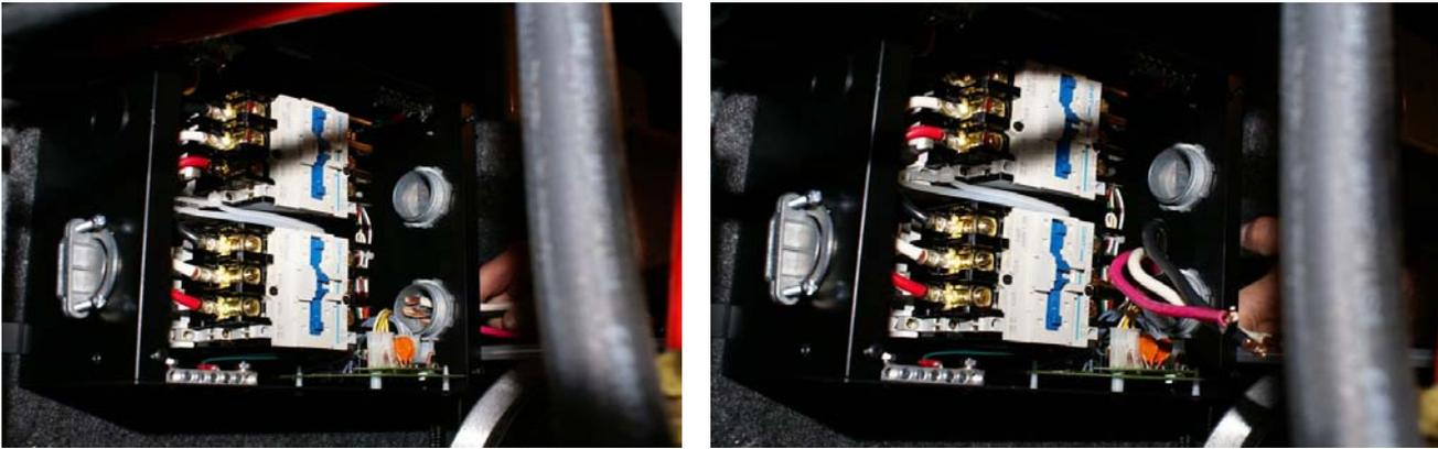
15. Insert the shore power cable through the right hand upper romex connector. Repeat the step #14 process on this cable with the exception that the bonding ground wire is Green colored instead of Bare Copper.
