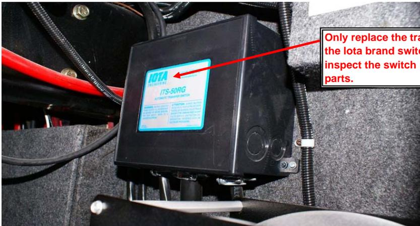
Only replace the transfer switch if it is the LOTA brand switch shown. You must inspect the switch prior to ordering parts.
