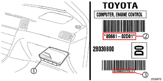
Locate the PCM (1) under the glove box compartment.
